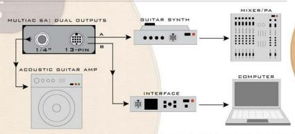
\*USE 1/4" OUTPUT THROUGH ACOUSTIC GUITAR AMP OR PA FOR OPTIMAL SOUND.
